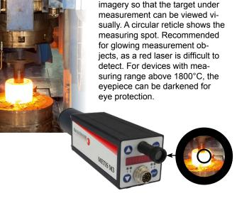
Laser targeting uses a red laser dot showing the center of the measuring field. At the focus point, the laser dot is the smallest and provides the sharpest image, so that the measuring distance for the smallest spot size can be easily determined.
